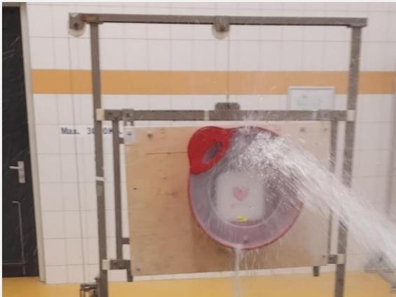
Image during IP X6 water test front
