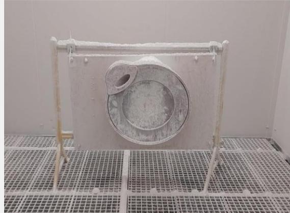
Image after IP 5X dust test
