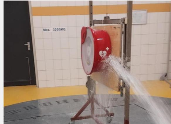
Image during IP X6 water test side
